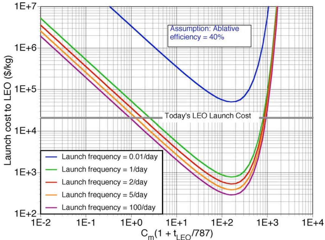
**Figure 2. Cost of laser launching 10 tonnes to LEO** using a repetitive-pulse deuterium-fluoride laser, figure adapted from ref. 17 to illustrate the importance of launch frequency.
