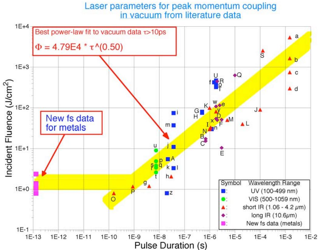
**Figure 3. Fluence required for optimum coupling and plasma formation** on a target in vacuum is a minimum across the entire range from 100fs to 100ps.
