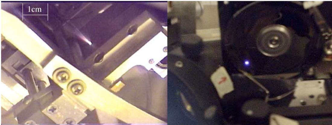
**Figure 4.** Jets from the ms-pulse (left) and ns-pulse microthrusters in vacuum [see, e.g., 12]. The ns-pulse jet was demonstrated in tests with a spinning laptop hard drive disk, and operated for 4 hours.
