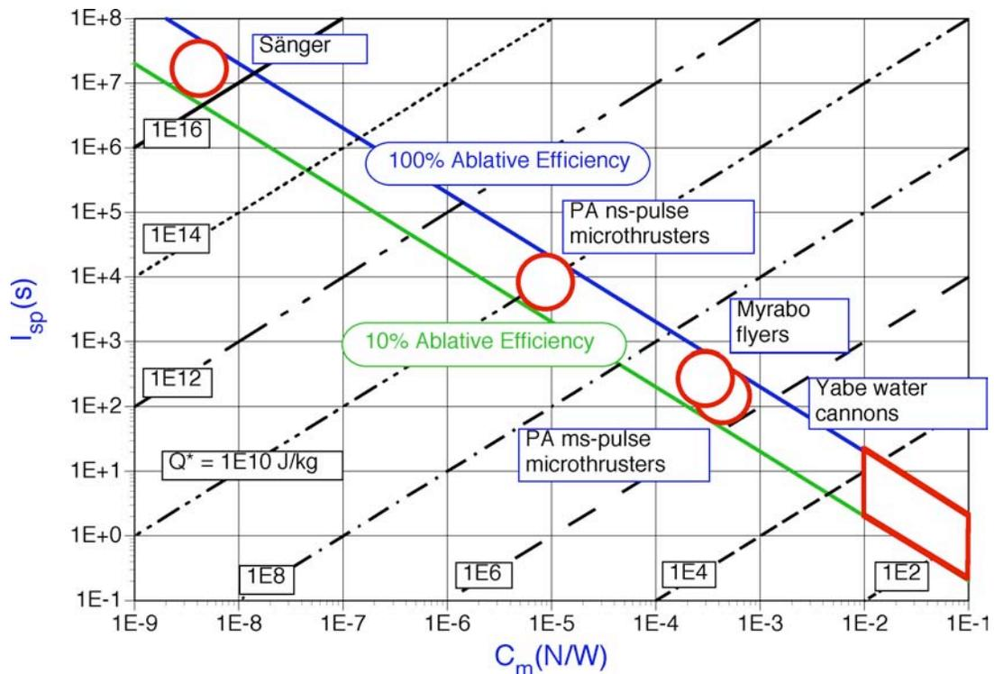
**Figure 1.** Specific impulse vs. momentum coupling coefficient for several types of photon-powered flyers. Lines of constant energy investment are shown.
